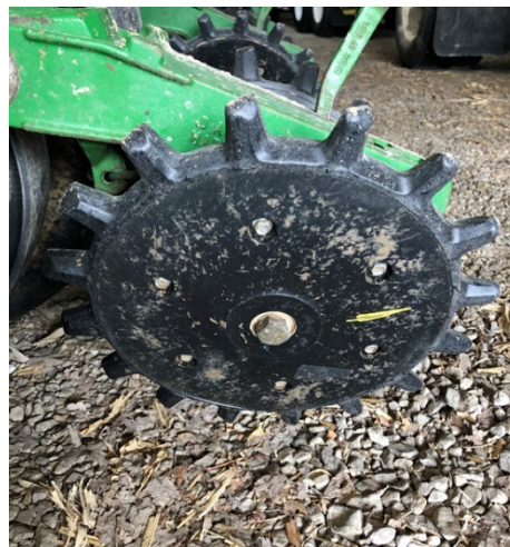
Figure 7. Closing wheel equipment modification for no-till corn and soybean planting.
